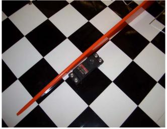
12. We recommend the use of a mini servo for throttle actuation. There is a pre-cut opening on the left interior rib for mounting the throttle servo. This opening is sized for a standard servo. We also supply a plywood mount for a mini servo (Hitec 225, etc.) that is to be glued into place if a mini servo is used. You may find it easier to mount the servo in the ply wood mount before gluing it into position.
