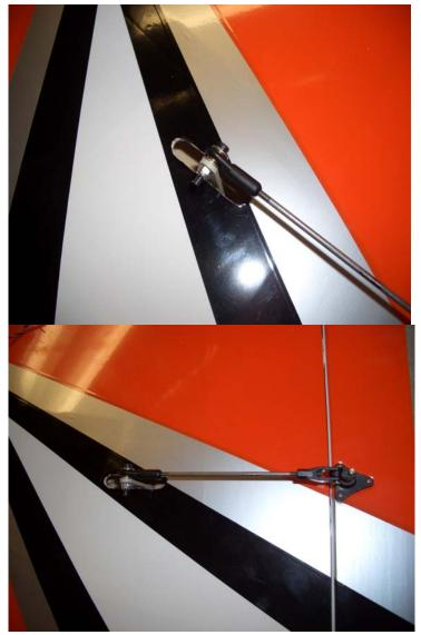
16. The rudder linkage assembles and is installed the same way. Screw in the control horn connector so that the linkage does not interfere with the movement of the elevons. Cut off the bolt that secures the rudder ball link flush with the top of the nut.
