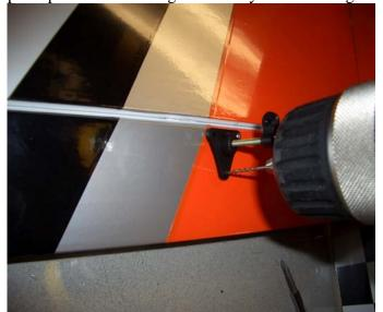
15. Thread a clevis onto one end of the pushrod and a ball link onto the other end. Secure the clevis to the control horn with the provided screw and secure the ball link to the servo arm with the 3mm bolt and nut. The distance from the hinge line to the pivot point should be the same as the distance from the servo output shaft to the location of the ball link on the servo arm for best mechanical set-up. Screw the connector down on the threaded horn to the proper position.
