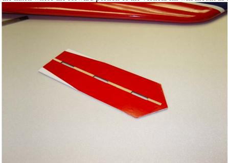
5. Glue the forward portion of the vertical fin to the hatch with 30 minute epoxy, making sure the fin is perpendicular to the top of the hatch. Trial fit before gluing and it is also a good idea to test fit the fin/hatch to the aircraft to be sure the tongue and groove portion is properly aligned with the fixed portion of the vertical fin.
