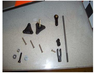
14. Use a straight edge aligned with the protruding servo arm to determine location for the elevon control horns to be mounted. Place the triangle shaped horn in place and drill through the control surface at the location of the 3 holes. Use the provided screws to secure the control horn to the surface and thread them into the base plate on the bottom of the surface. Make sure to position the horn so that the pivot point of the linkage is directly over the hinge line.
