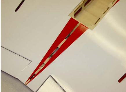
3. The vertical fin has a series of tabs and notches to add rigidity and allow for easy alignment of the vertical fin. Trial fit the fin in place to insure proper alignment. Once satisfied glue the fin in place with 30 minute epoxy. Check from several angles to make sure the vertical fin is properly aligned and square to the wing.
